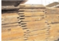
above: reusable wood timbers salvaged from demolition site
